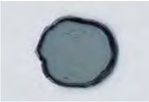
打开 进行70℃×1h加热后 热循环试验 25循环 Oven-heated to 70°C for 1 h + 25 cycles
